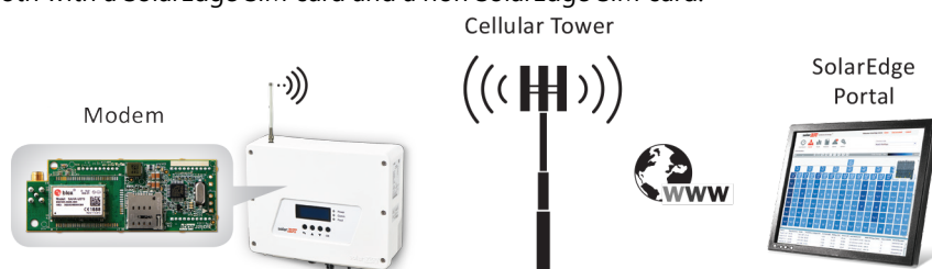
Figure 16: Low bandwidth mode, single device, cellular modem connection
