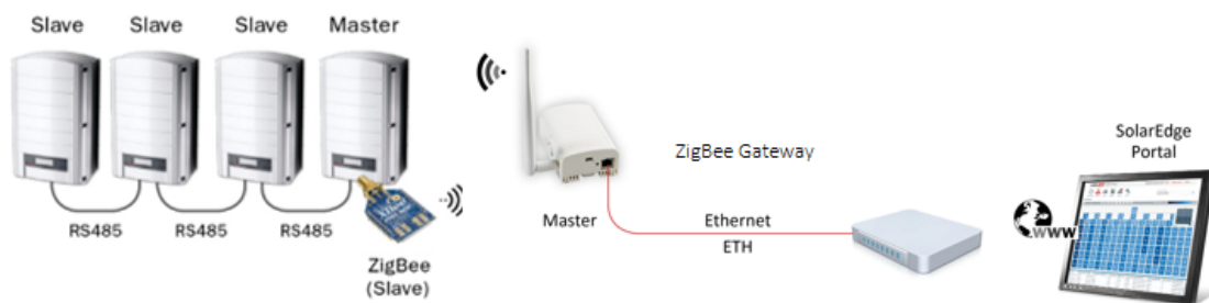
Figure 13: Multiple devices, RS485 bus , ZigBee server connection
